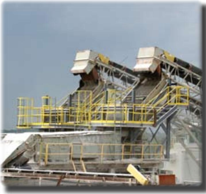
Astec Mobile Screens offers the PEP 6' x 12' series of Vari-Vibe® high frequency screens in single, double and triple deck screen configurations in stationary applications. Other configurations are available in portable structures, as well as mobile screening plants depending on model.
